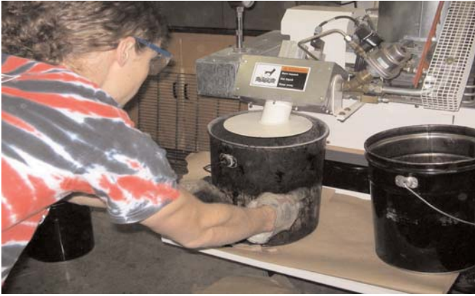
Figure 36. Introducing foamed asphalt to mixing bucket.
