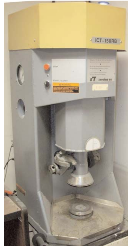
Figure 5. Gyratory compactor with shear stress measurement.
