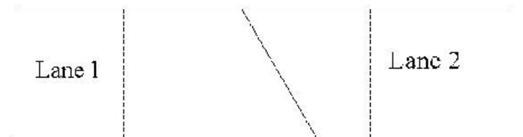
Figure 3. Core centered on the longitudinal joint
