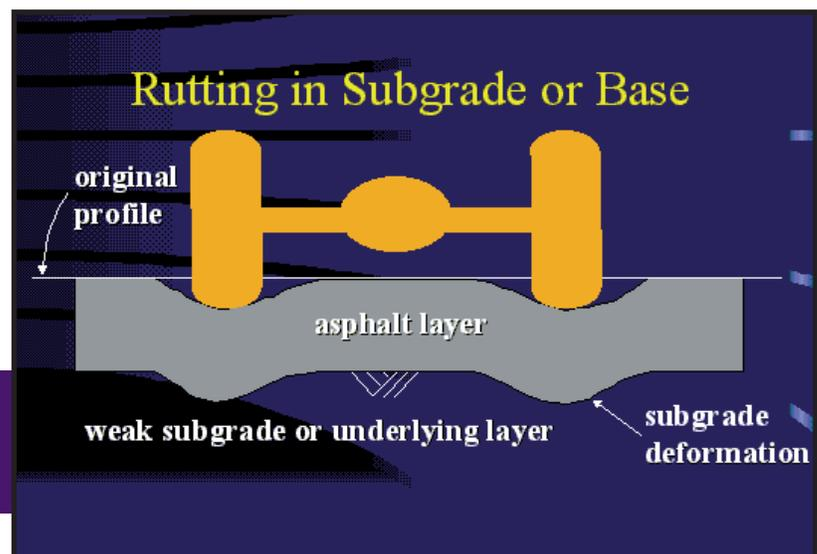
Figure 1: Rutting in the subgrade; a weak subgrade or base will expedite damage in all pavements.
