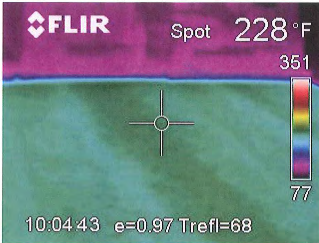
FIGURE 6 Thermal Image of Sasobit Mat (Picture courtesy of Becky Smith)
