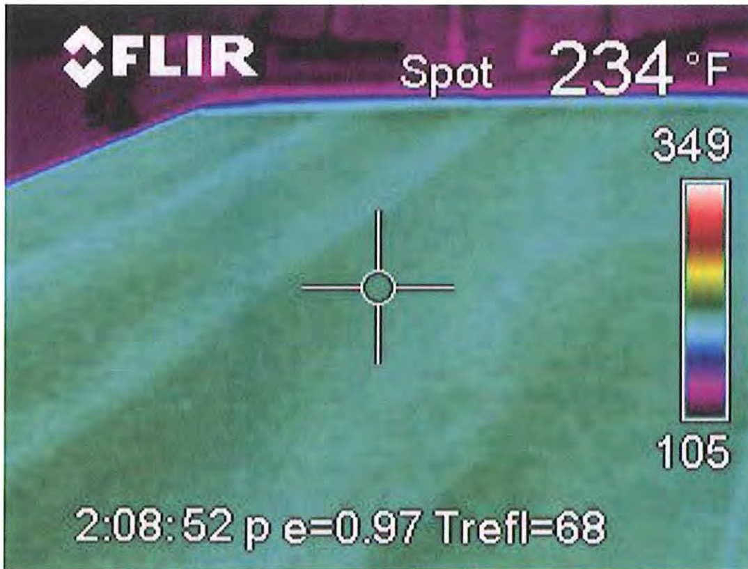
FIGURE 2 Thermal Image of Astec DBG Mat (Picture courtesy of Becky Smith)
