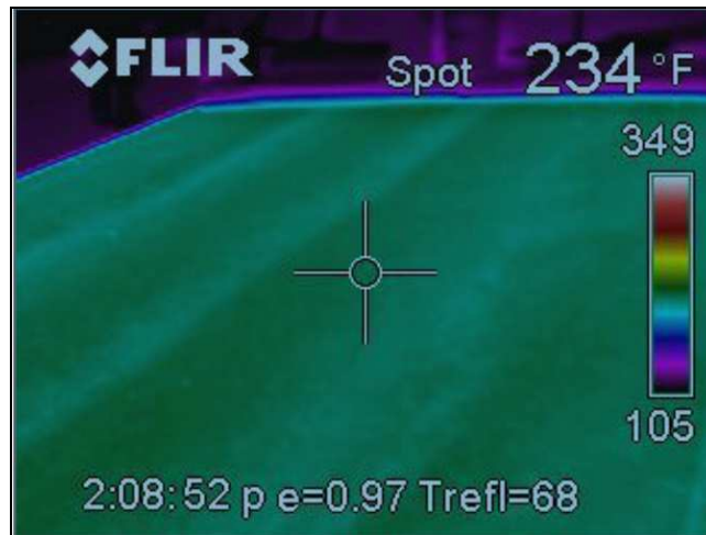
Figure 5.1: Thermal image of WMA section showing consistent mat temperature.
