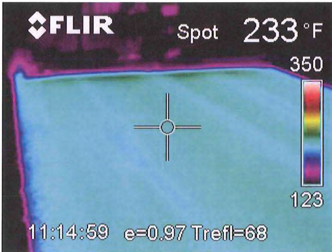
FIGURE 5 Thermal Image of Evotherm DAT Mat (Picture courtesy of Becky Smith)
