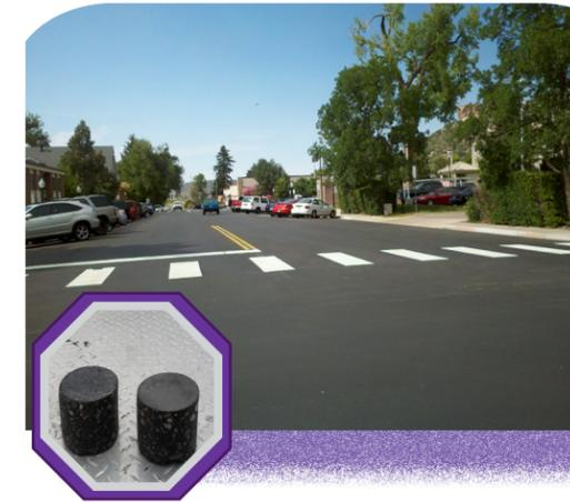
Specifying the right asphalt mixture for the right application is a very important consideration as it relates to long term pavement performance. Designing a mixture to be durable and able to withstand surface oxidation and weathering needs to be balanced with having stability to withstand rutting (ie. permanent deformation). There are
