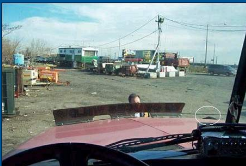
Driver's field of view inside of a tanker truck. Can you see the workers in front of and directly to the right of bug shield? (circle)
