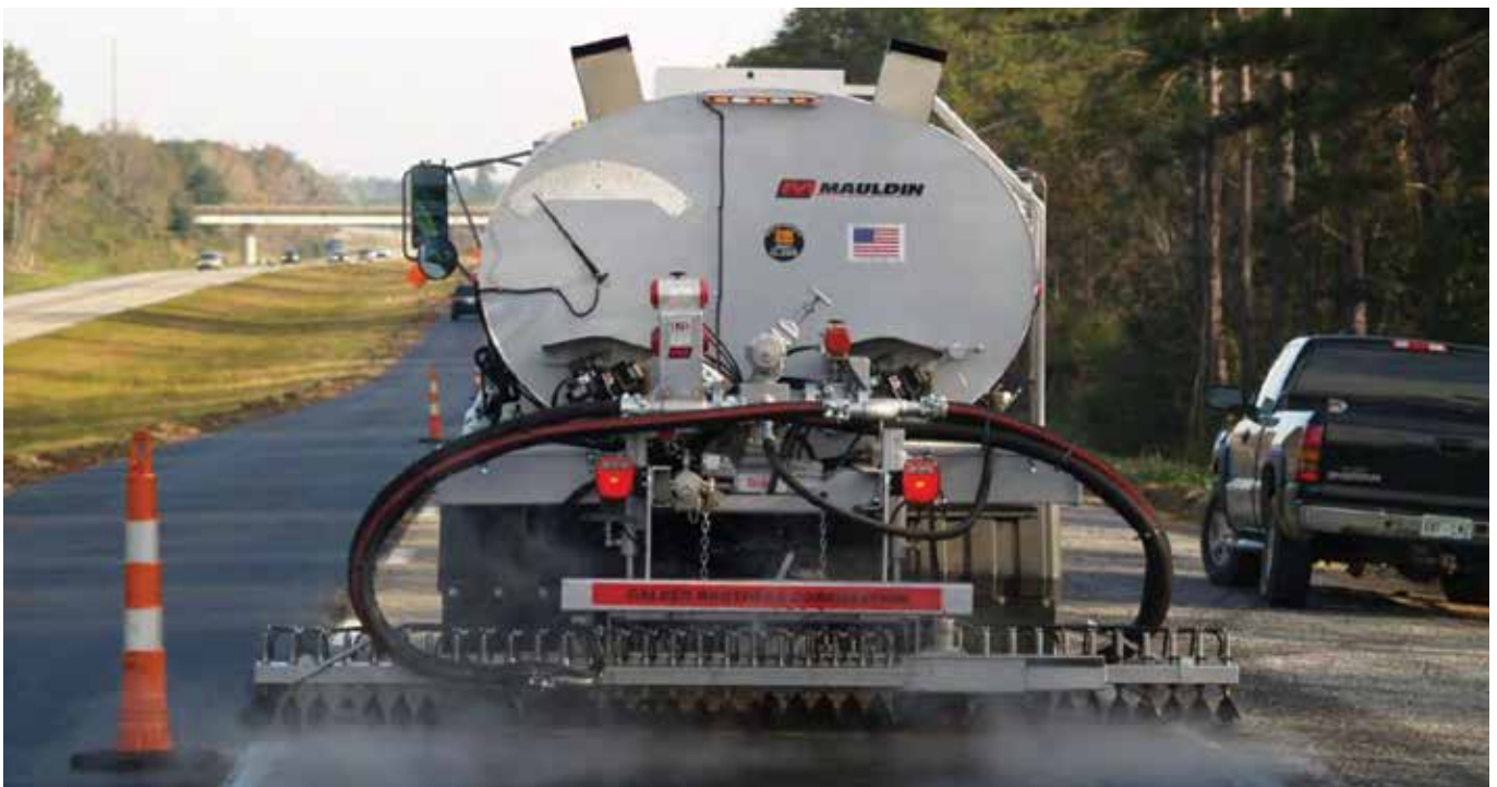
Figure 3-4. Spray Bar on Distributor
