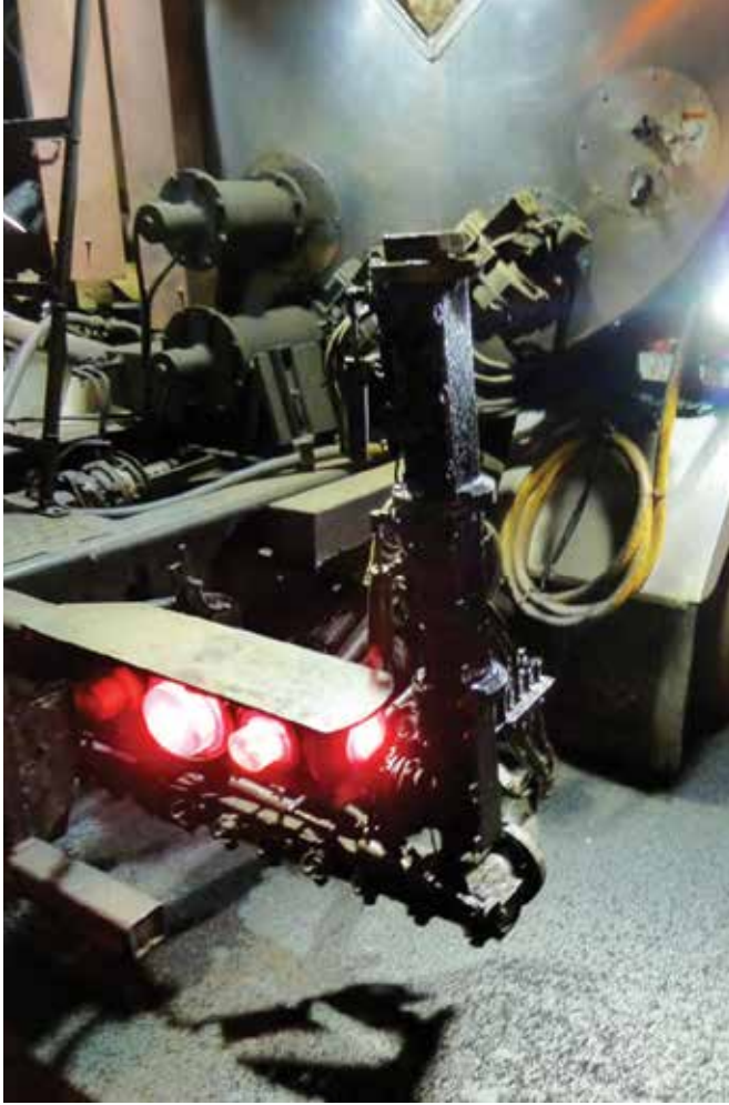
Figure 3-5. Folded Spray Bar Configuration
