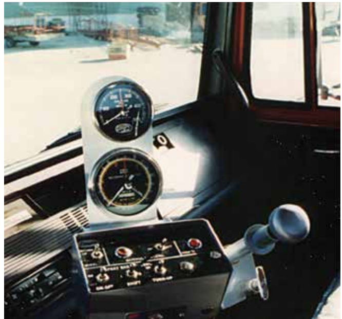
Figure 3-2. Tachometer-Style Distributor Control
