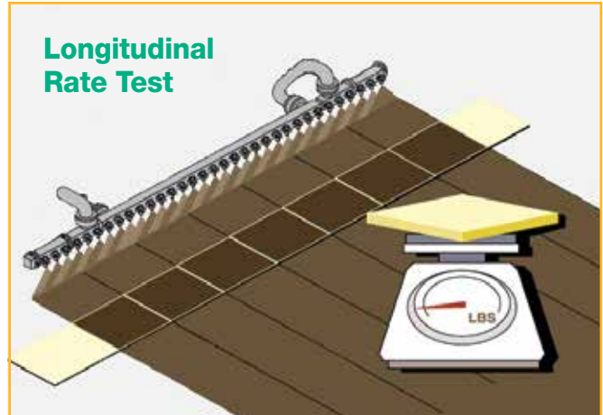
Figure 3-15. Calibration of Tack Coat Distributor
