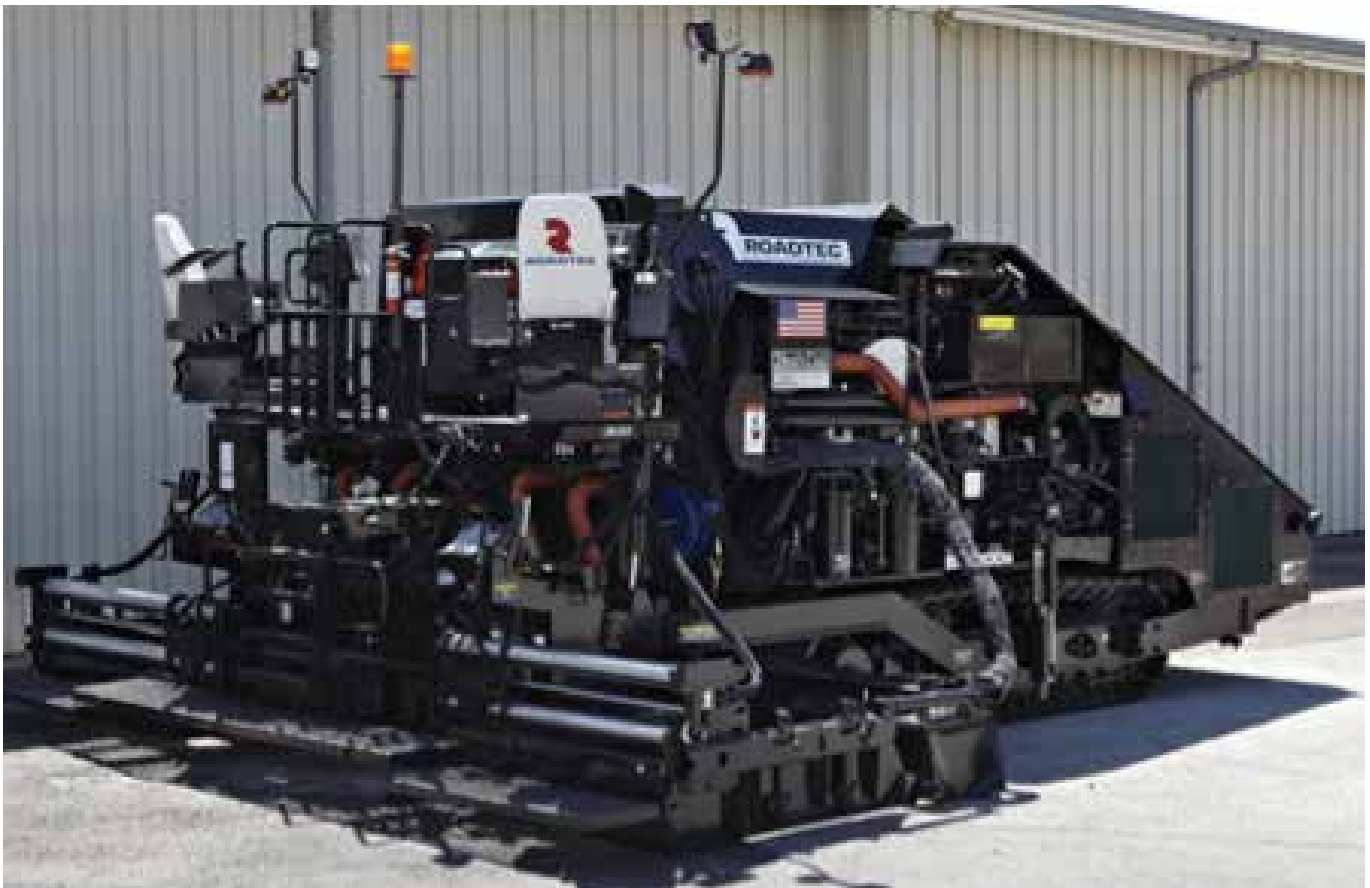
Figure 10. Roadtec SP-200 Spray Paver
