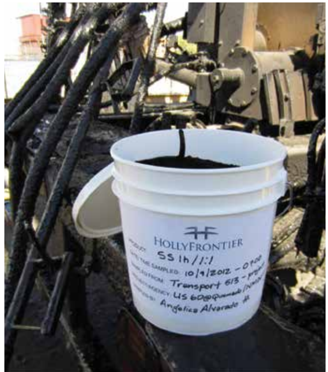
Figure 2-2. Sample of Asphalt Emulsion
