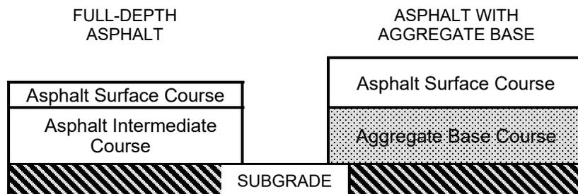
The minimum thickness recommendations are suitable for the cars and light trucks plus the occasional heavier service and delivery trucks normal to the single unit residence.
