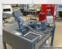
Lab Test (Hamburg Wheel Tracker)
