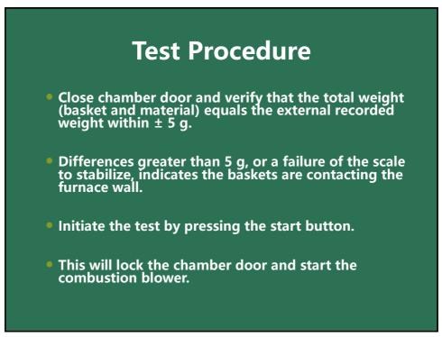
Allow the test to continue until the stable light and audible stable indicator indicate the test is complete (the change in weight is less than 0.01% for three consecutive minutes).
